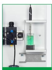
The onboard maintenance station allows for onsite calibration, cleaning, and consumable replacement, maximizing convenience.
